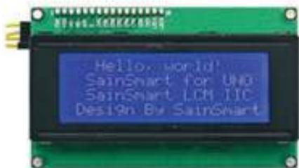
Figura 12. Display LCD IIC/I2C/TWI
