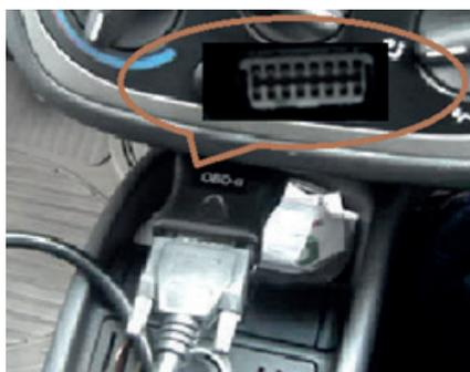
Figura 3. Conector OBDII
