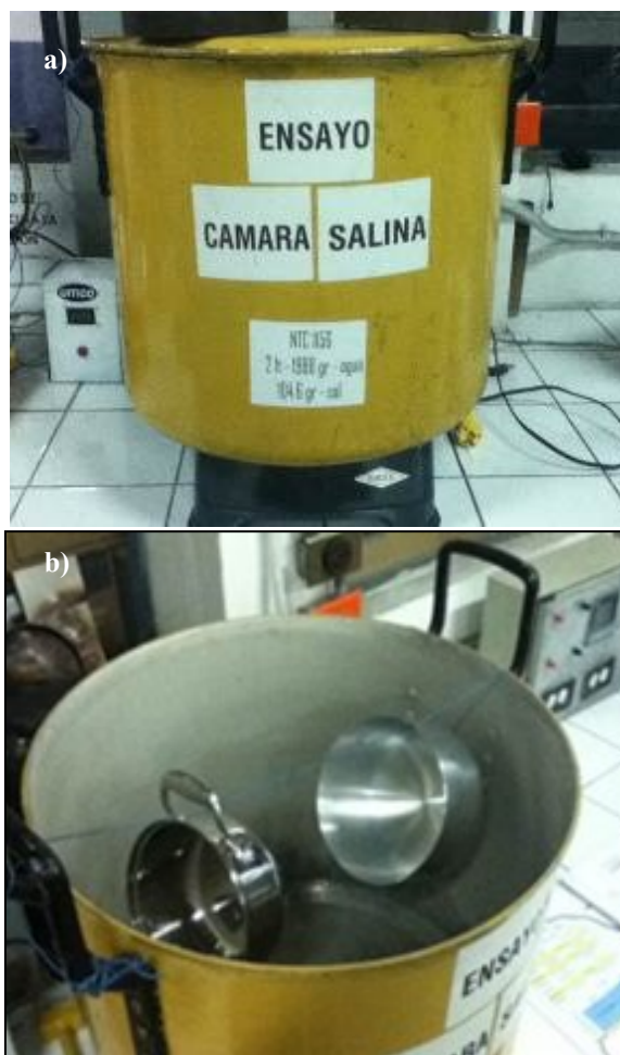
Fig. 1. a) Image of the salt spray chamber for material corrosion test. b) Image of two pots suspended in the salt spray chamber.
