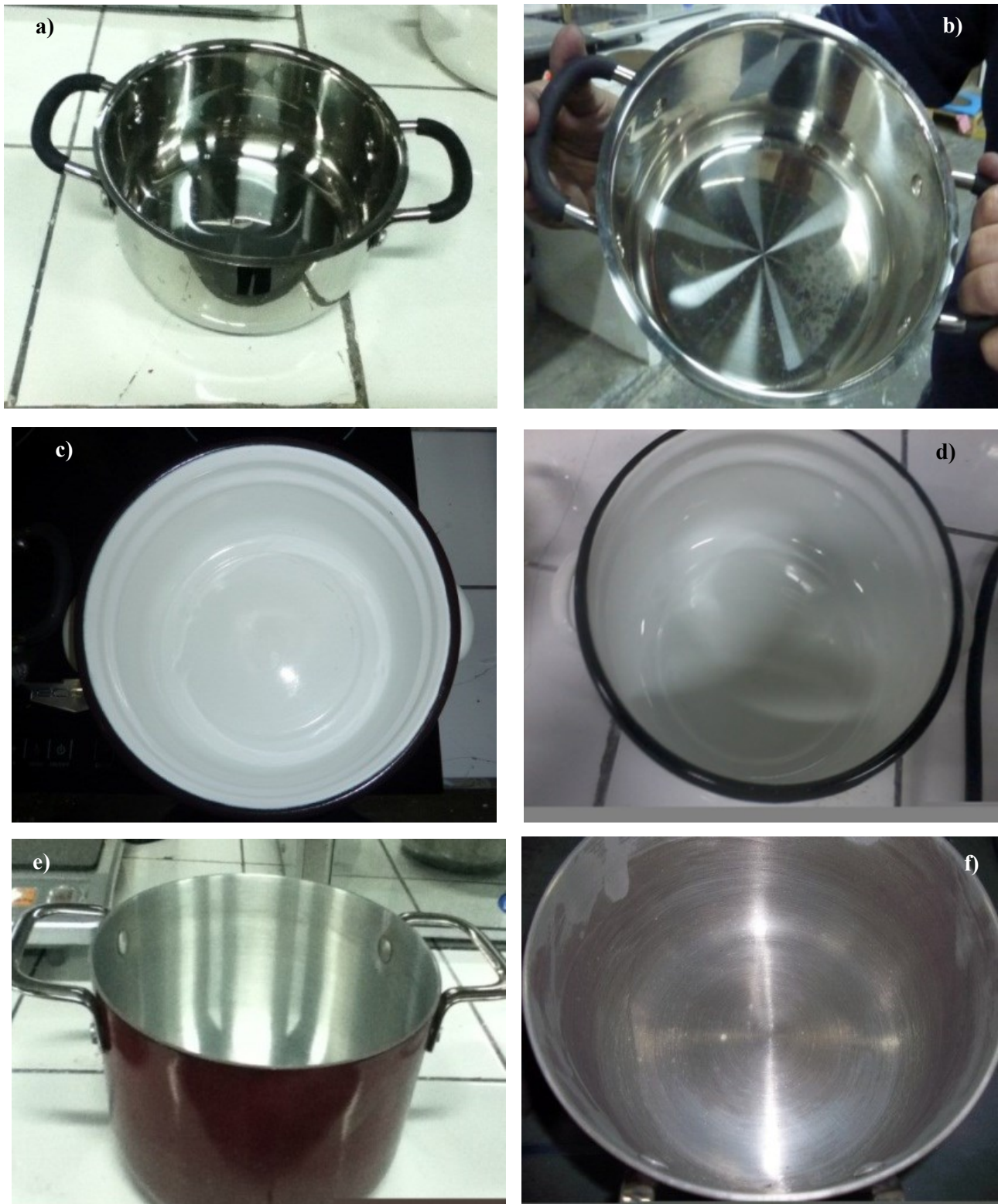
Fig. 2. a) y b) Images of stainless steel cookware before and after corrosion resistance in a salt spray chamber test, c) y d) Images of cast iron pot before and after corrosion resistance in a salt spray chamber test, e) y f) Images of aluminum body pot before and after corrosion resistance in a salt spray chamber test.
