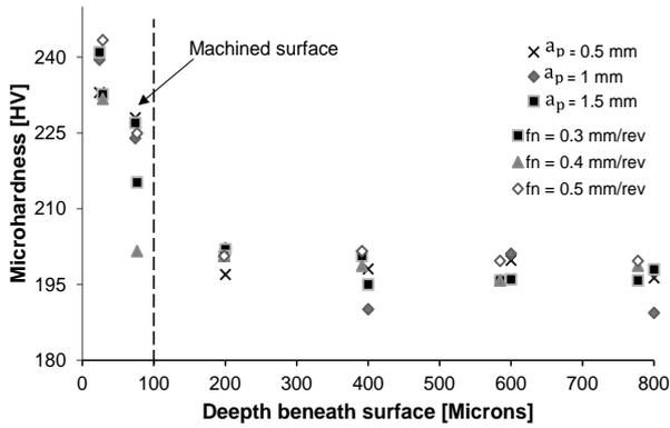
Fig. 3. Microhardness on AISI 1018 machined surface.
