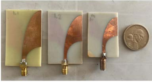
Fig. 13. Implementation of Vivaldi antennas 1.1, 1.2, and 1.3.
