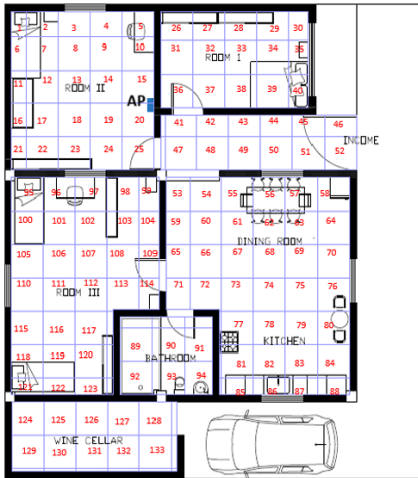
Fig. 4. WiFi network measurement points: implementation in SketchUp.
