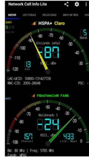
Fig. 8. Power measured at 2 meters from the router.
