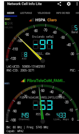
Fig. 6. Network Cell Info Lite application for operating band determination.
