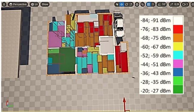
Fig. 13. Mapping of Received Powers.
