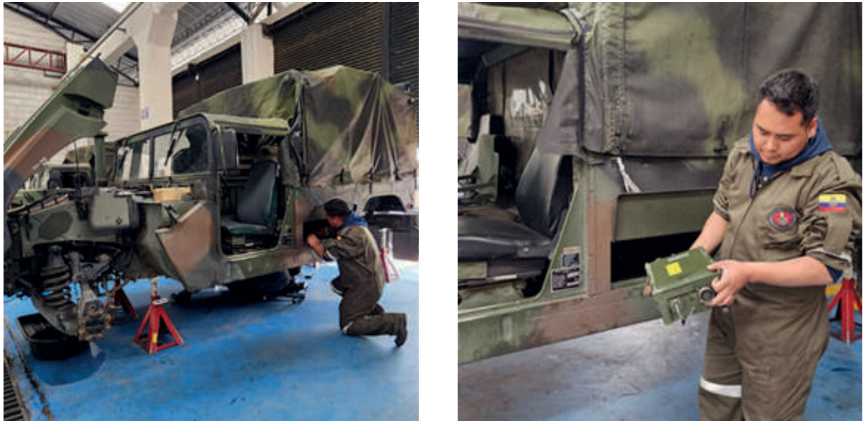
Figura 1: Transmission Control Module Assembly Allison 4l80E HMMWV TCM.
